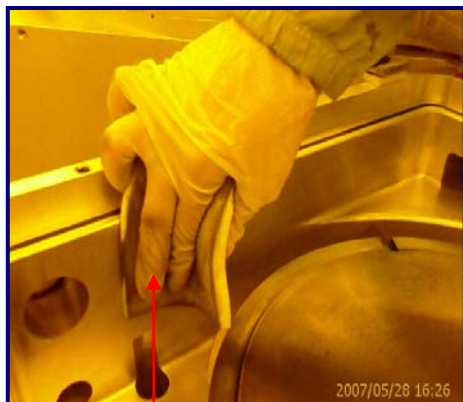
Fig 21: Wiping Degas Chamber wall
