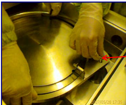
Fig 69 & 70: Replacing lift ring back into Degas Chamber (1 st & 3 rd generation shown)
