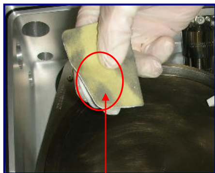
Fig 14: ScrubPAD loaded with deposition
