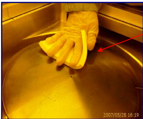
Fig 11: UltraSOLV® Sponge wiping loose residue on surface of Degas Heater
