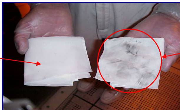
Fig 48a: Current fab wiper after completely wiping Degas Chamber
