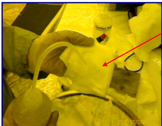
Fig 60: Saturating MiraWIPE® with IPA
