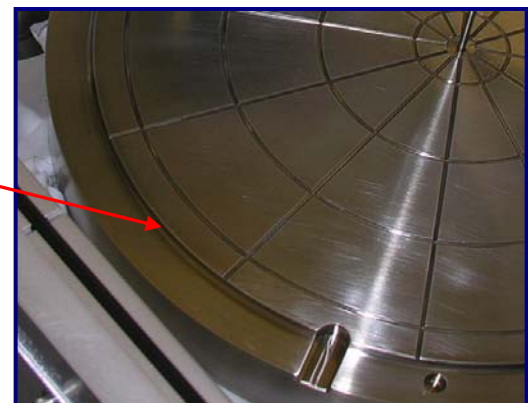
Fig 33 & 34: Process build-up on the edge of heater missed during initial scrub of Degas Chamber
