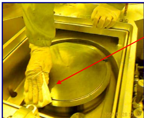
Fig 64, 65 & 66: IPA saturated MiraWIPES® wiping down Degas Chamber
