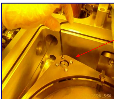
Fig 1 & 2: Removing Degas Heater lift ring
