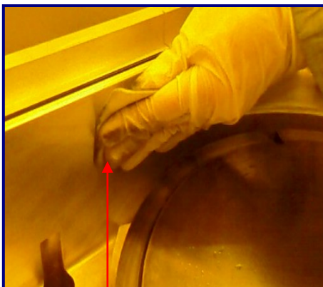
Fig 22: Scrubbing top portion of Chamber walls
