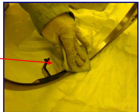
Fig 55 - 58: Scrubbing Degas Chamber lift ring on workstation
