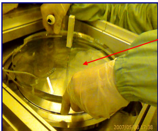
Fig 71 & 72: Aligning to Degas Heater lift ring using AMAT's alignment fixture (1 st & 3 rd generation shown)
