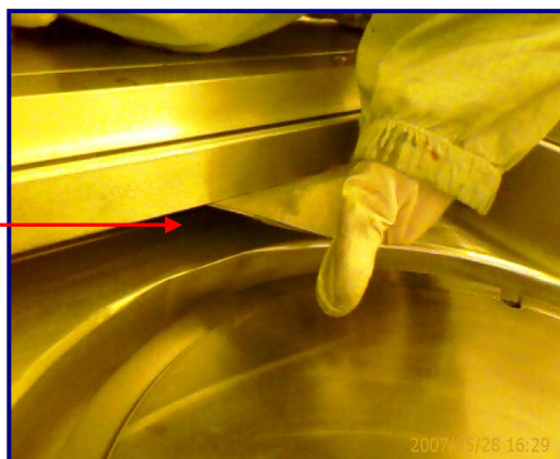
Fig 26 & 27: Scrubbing top and bottom portion of slit valve area
