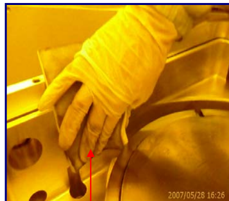
Fig 23: Wiping Degas Chamber wall clean
