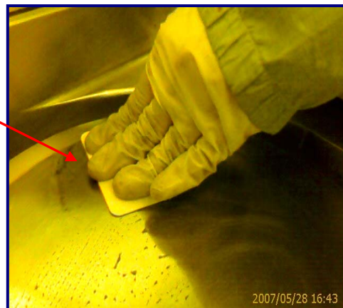
Fig 29 & 30: Second 360 Grit Diamond ScrubPAD scrubbing buildup missed on initial scrub of Degas Chamber
