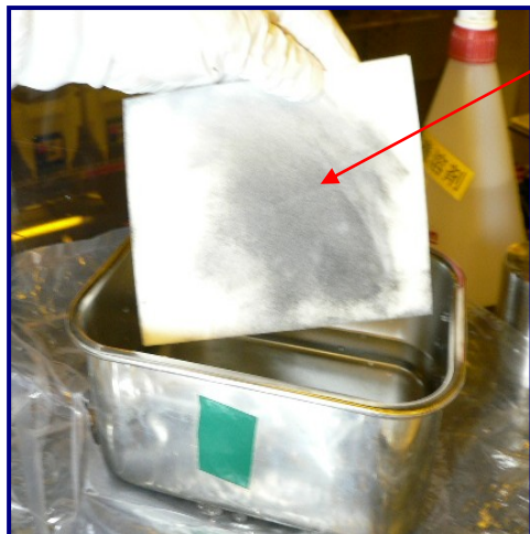
Fig 10: UltraSOLV® Sponge loaded with deposition
