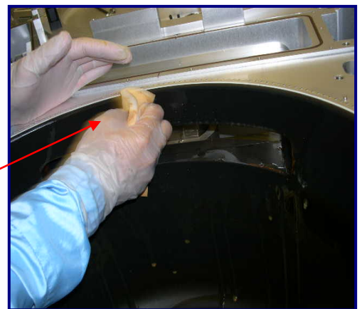
Fig 3: UltraSOLV ® Sponge wiping Metal ETCH Chamber, 90% of deposition removed
