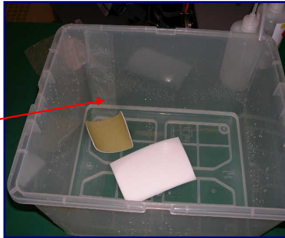
Fig 1: Container of DI water with ScrubPAD and UltraSOLV ® Sponge
