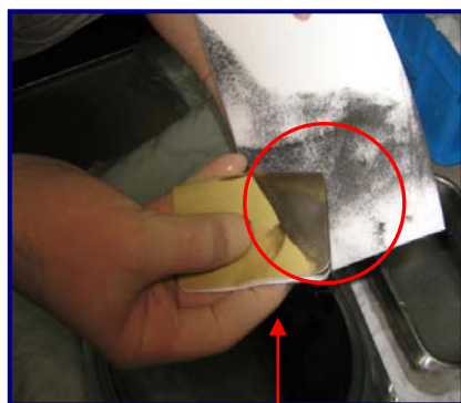
Fig 7: ScrubPAD loaded with deposition
