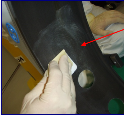
Fig 5 & 6: Lightly dampened 800 Grit Diamond ScrubPAD scrubbing chamber liner; keep slightly moist with DI water
